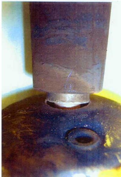
(ER v.4 805, Vanderlinde cylinder, failing at the brazed joint (Declaration of J. Vanderlinde at ER vol.2 354)
