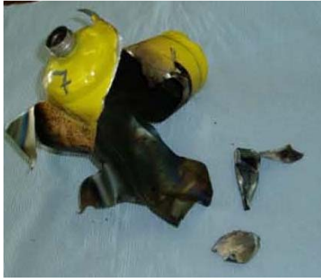
(ER vol.2 269 - an "Exploded" MAPP cylinder from British Report)
